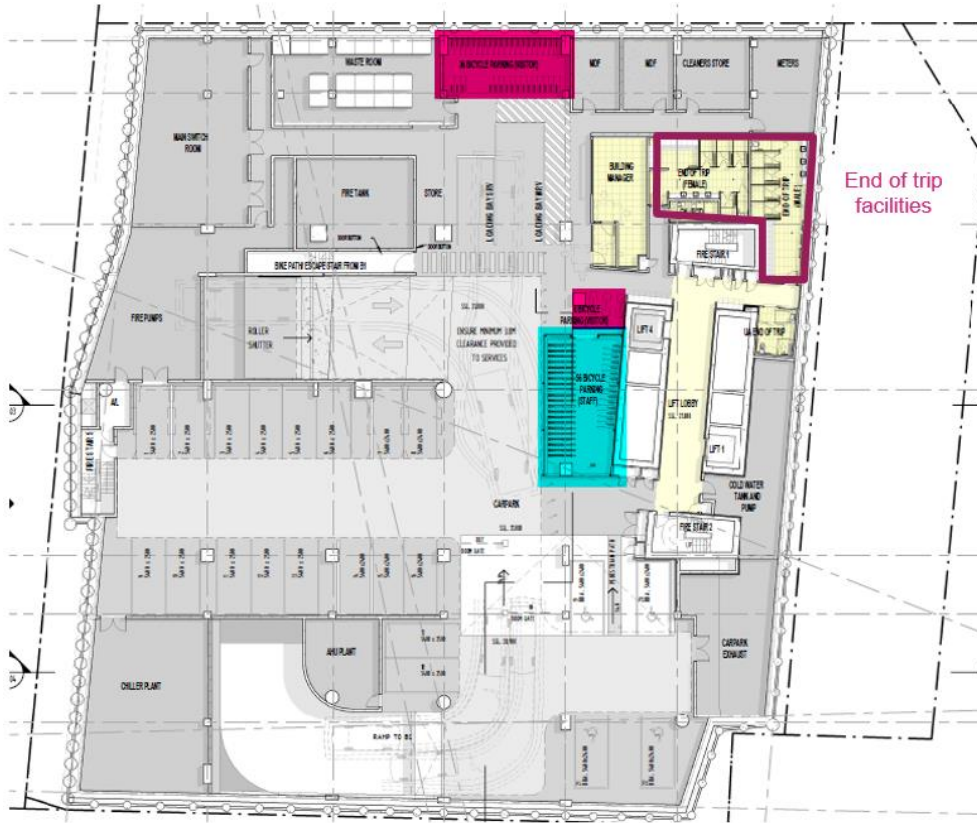
Figure 12: End-of-trip facilities within basement
